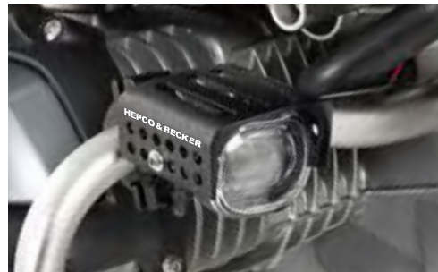
LED Flooter - horizontal mounting
