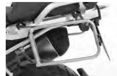
Side carrier - firmly bolted Surface-blasted, electro-polished side carrier
